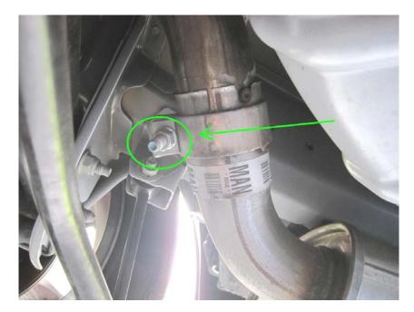
3. Next, you need to remove the bolts that are currently holding the (2) muffler hangers to the under body of the car. **NOTE:** Work back to front when dissembling and front to back when reassembling. This will make it easier to remove the muffler and get the new axle-back installed centered in the exhaust cutout on the bumper.
