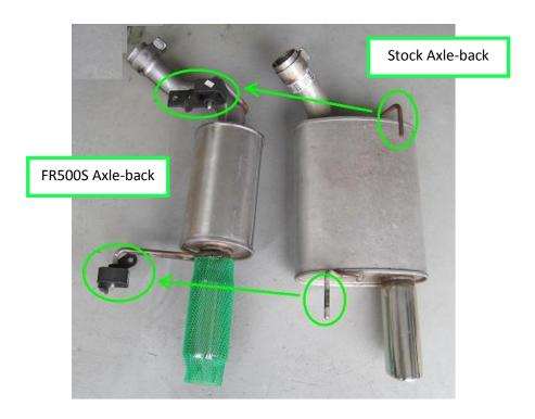
6. Next, insert the exhaust pipe end of your new exhaust into the mid-pipe. You may need a friend or a well-placed knee to keep the axle-back up in position until you have the chance to bolt it in. It may take a little elbow grease to get it fully into the mid-pipe. There is a set screw that you can use as a reference point to ensure proper positioning.
