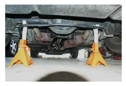
4. Use a 12mm wrench to remove the (4) bolts from the rear u-joint and rear differential.
