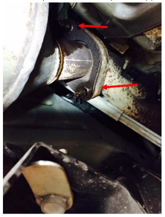
**8.** After you are done removing the 4 nuts (2 nuts on each side) slide your H-pipe off. It may be hard to get off so just wiggle it around until it slides off. Now it's time for the installation of your new X-pipe.
