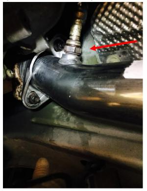
**9.** Now check for exhaust leaks. You can check for exhaust leaks by starting your car and putting your hand close by the connections of the rear pipes and the crossover pipe, the connections between the down pipes and the crossover pipe, and also the connections between the down pipes and the headers. If you feel any air coming out of those connections be sure to tighten the specific connection where you have a leak.
