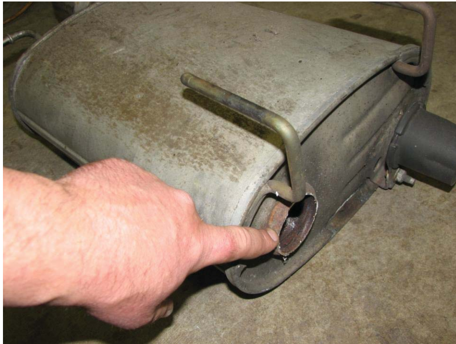
Figure 1: Cut off factory mufflers here
