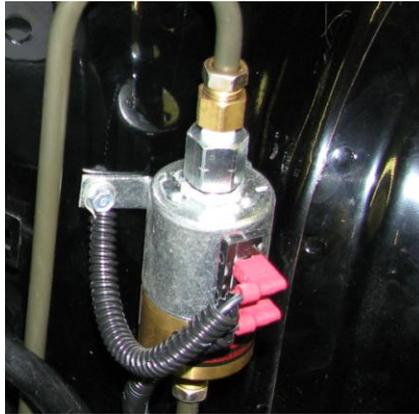
**Figure 5: Installation of ground wire**
