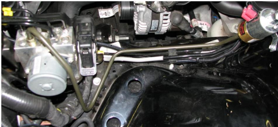
**Figure 4: Proportioning valve to solenoid line routing**
