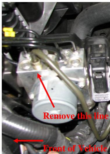
**Figure 2: Removal of line in proportioning valve**
