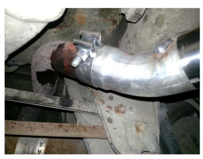
**Step 9**. Replace the two bolts in the hanger nearest the rear of the car. Then replace the one bolt in the hanger nearest the mid pipe (REMEMBER the hanger you removed in step 3 is
