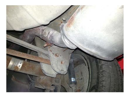
**Step 5**. Locate the final hanger closest to the exhaust tip and using a 1/2" socket unbolt the hanger from the car. NOTE: This hanger has TWO bolts that must be removed see figure 4
