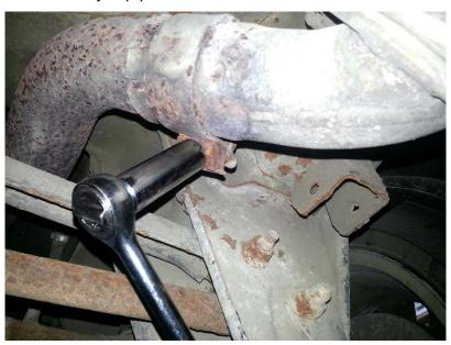
**Step 3**. Find the metal hanger that is curved around the back pipe of the muffler (in between the mid pipe and actual muffler) which is welded to the muffler. Using a 1/2" socket wrench unscrew both of the bolts connecting the hanger to the car. This hanger will NOT be used when installing the new muffler.
