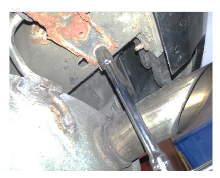
**Step 4**. Moving from the front of the car to the back locate the next hanger and unbolt the hanger from the car using a 1/2" socket wrench. NOTE: This hanger only has one bolt connecting it to the car.
