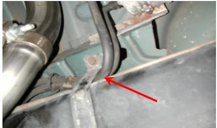
14. Please view photo below of suggested clearance of passenger side tailpipe to the passenger side of the gas tank.
