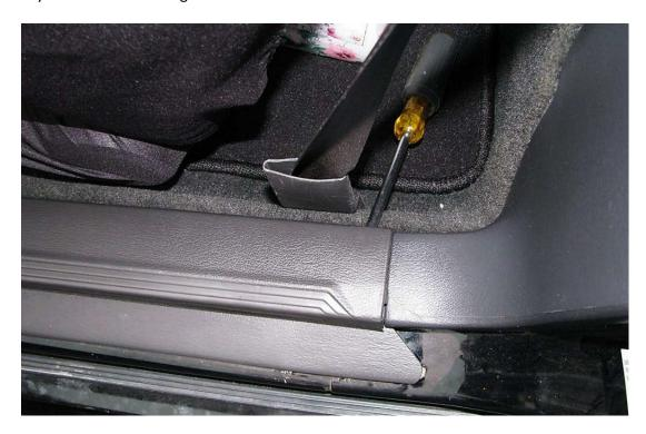
2. Pry off the (3) metal retaining clips with the screwdriver and put aside. You will be reinstalling these as well.
