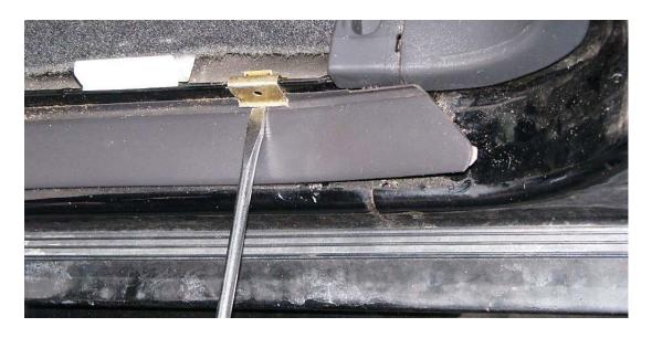
3. Starting at one side, gently slide the screwdriver along the underneath of the entire OEM sill. You may need to lightly pryit up if you feel resistance. You no longer need this piece when installing the new sills.
