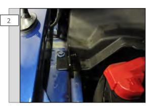
Install bracket marked P-L using factory fender bolt as shown.
