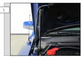
Pop the ends of the strut over the ball mounts on the brackets. Repeat steps 1-5 for drivers side. *(do not slam hood shut yet)* Check bumper/fender alignment by slowly lowering the hood. If okay, remove factory prop rod and enjoy.
