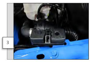
Remove the square rubber bushing from the bracket and cut ½" from the center of it. Place the two halves of the bushing onto the top side of the bracket as shown.
