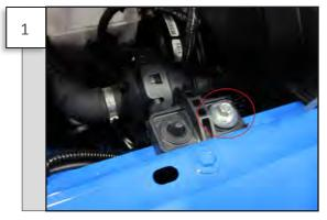
Remove the bolt holding the canister bracket to the inner fender. Also remove the factory u-nut from the fender for reuse.
