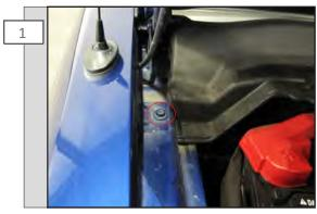
Prop hood open and remove the fender bolt shown below.
