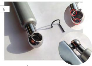
Remove the retaining clip. Place strut on the ball stud. Then reinstall the retaining clip.
