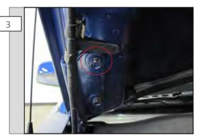
Making sure the hood is properly supported by the factory prop rod, remove the forward most bolt on the hood hinge.
