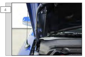
Loosen the rear most bolt on the hood hinge just enough to slide the larger bracket (marked P-U) in between the hood hinge and bolt. **(do not install the bracket between the hood hinge and hood)** Re-install/tighten bolts to secure bracket.
