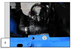
Re-insert the metal bushing (removed in Step 2) into the bottom right side of the bracket and re-install assembly on the bottom side of the inner fender using the original hardware (removed in Step 1).
