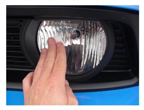
2. Peel the backing from the adhesive tape and place the round portion of the cover between the fog light and grille as shown.
