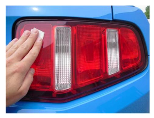
2. Peel the backing from the adhesive tape on the light cover and position over factory tail light, making sure that the lens is fully covered. When you are satisfied with the positioning of the cover, firmly press down on the cover to seat the adhesive tape. Repeat instructions for opposite side cover to complete the installation.
