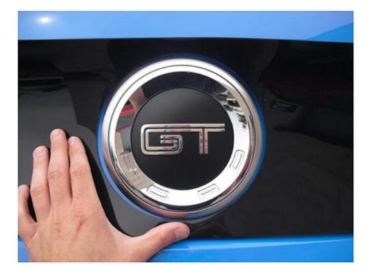
3. Once the panel is centered and the edges are covering all painted surfaces of the decklid, firmly press down on all areas of the panel to fully seat the adhesive.
