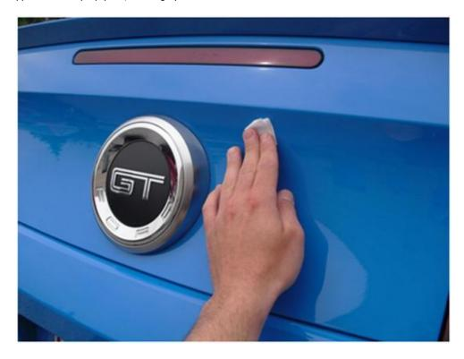
2. Peel backing from adhesive and place the cover over the decklid, using the center emblem as a guide.
