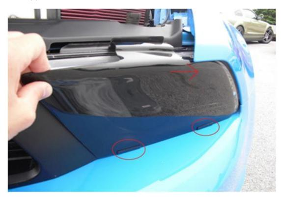
2. Once the light cover is secured under the factory headlight and fender, push the upper retaining clip over the headlight as shown. Repeat instructions for opposite side cover to complete installation.
