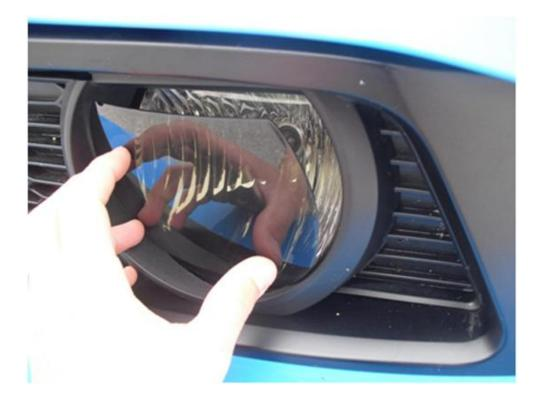
3. Once the cover is secured between the fog light and grille, firmly press down on the cover to fully seat the adhesive. Repeat instructions for opposite side to complete the installation.
