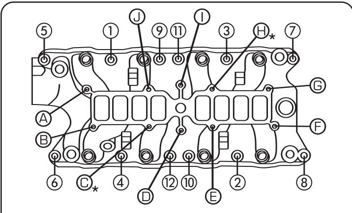
Intake Manifold Tightening Sequence and Upper Plenum to Manifold fastener locations
