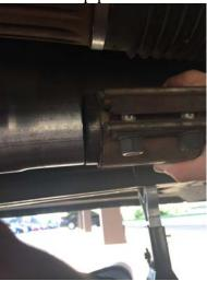
15. Clamp the band clamps to the new x-pipe using ratchet and 15mm deep well socket
