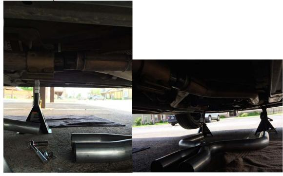
10. Using the reciprocating saw, cut the factory mid pipe off at the indicated markings
