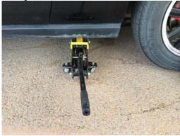
19. Remove the jack stand under the rear of the vehicle
