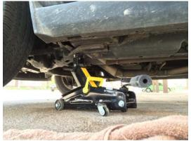
6. Mark spot of oem band clamp for reference during re-installment
