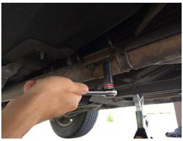
8. Following the provided instructions, measure and mark 9 in.  $-\,8$  in. back from the catalytic convertor
