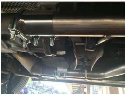
14. Due to my mishap previously stated, I had to get some pipe adapters to fit the space between the new x-pipe and the over axle pipe.
