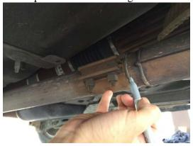
7. Remove the two 15mm bolts on the band clamp using a breaker bar and a 15mm deep well socket
