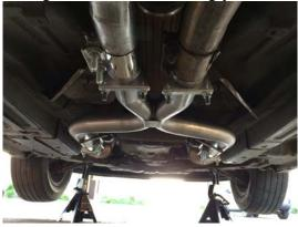
17. Once all connections are secured, jack the front of the vehicle and remove the front jack stands
