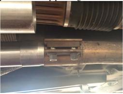
16. Inspect connections and tighten all bolts accordingly
