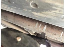
11. Using a drill and a deburring tool, deburr the cut portion of the factory mid pipe to promote a good seal
