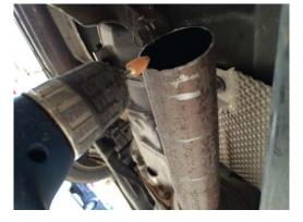
12. Thoroughly inspect the newly deburred factory mid pipe for loose burrs
