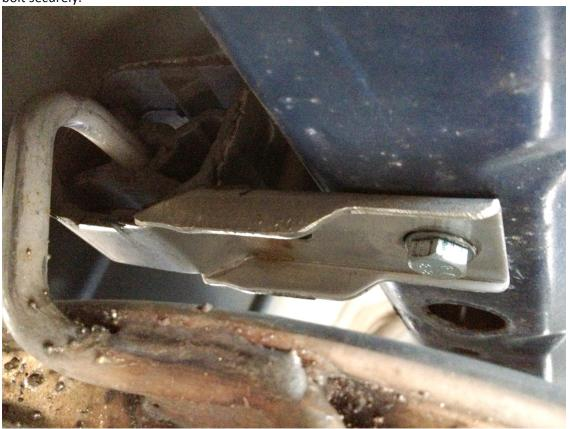
**13.** Tighten rear bracket bolts using a ½ socket with extension if needed.
