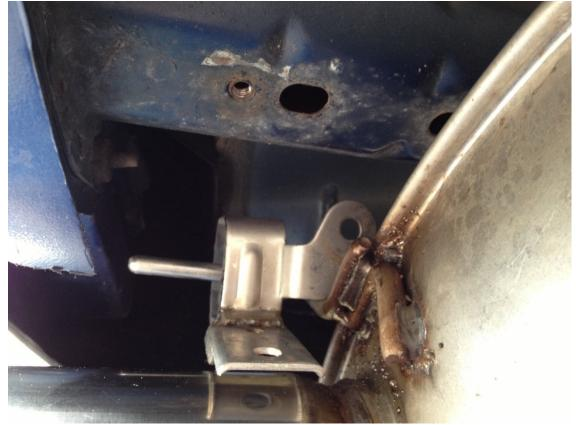
**9.** Proceed to install exhaust muffler pipe to intermediate pipe. It may require some wiggling and pushing until fully seated. Do not tighten 5/8 nut just yet leave loose for adjustments.
