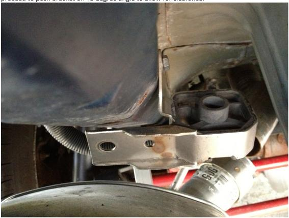
8. Install second rear bracket on muffler hanging rod above muffler tip.
