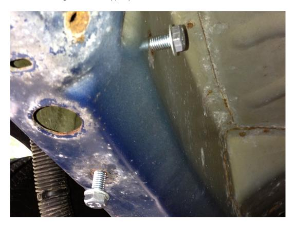
7. To install muffler first install front bracket with frame side rail bolt hand tighten only using a ½ socket then proceed to push bracket on 45 degree angle to allow for clearance.
