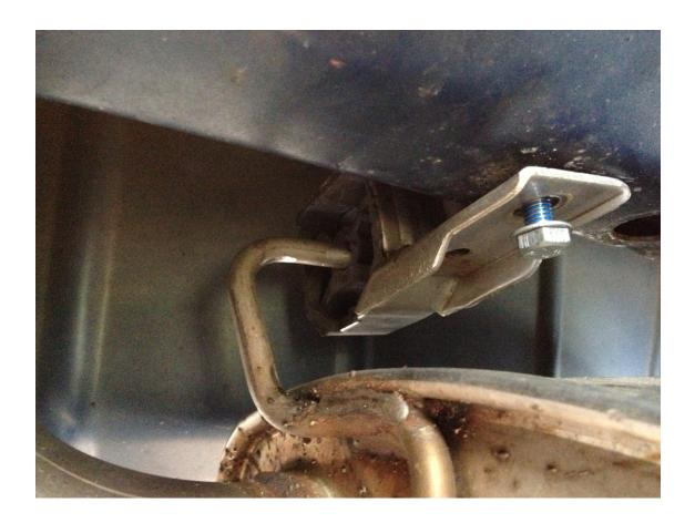
**11.** Proceed to second rear bracket, pushing up on the muffler tip; loosely attach both 8MM bolts by hand.
