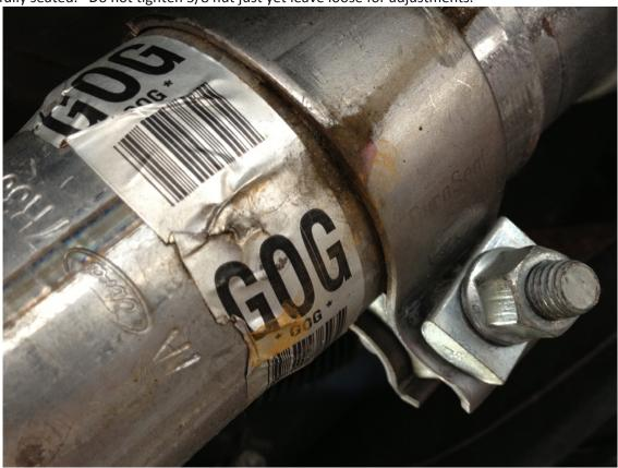
**10.** Push the muffler up and swing your front bracket down to slip over hanging rod. Install bottom nut in bracket and leave loose.
