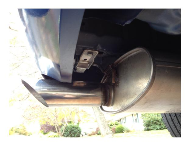
**NOTE:** To adjust for height your muffler has to be removed from vehicle. You should allow for ¼ gap for spacing to prevent damage to plastic bumper cover due to movement while driving.
