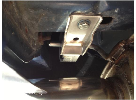
**14.** After tightening down all four bracket bolts you may adjust muffler alignment left or right. Twisting muffler body left or right until pipe coming rear is 90 degree and straight.
