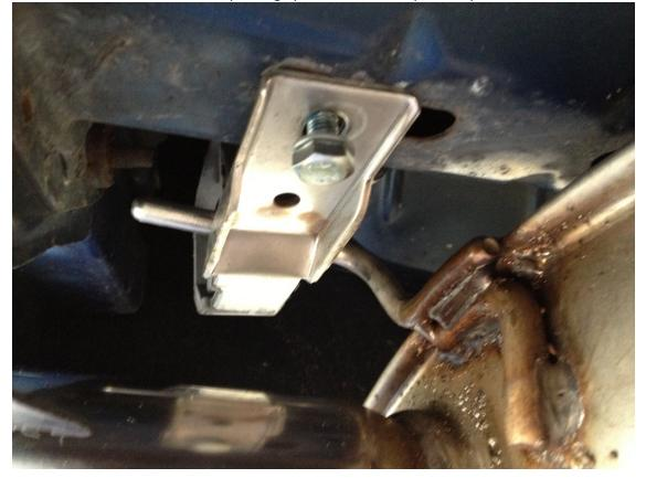
**12.** Start by tightening the front bracket bottom bolt using a ½ wrench to 18 ft. lbs. Then tighten side frame rail bolt securely.
