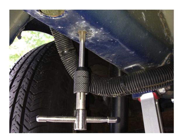
**5.** After tapping both front and back bottom frame rail bungs proceed to tap inner side rails using 8MM x 1.25 tap. Your T-handle will not fit on side frame rail located next to the spare tire wheel well. I found best to use ¼ wrench to turn tap or you may use an adjustable wrench.
