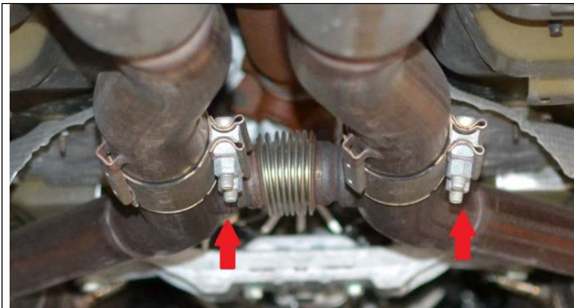
Clamps to remove to separate intermediate pipes from H-pipe
