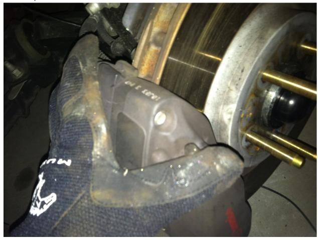
3. Thread the two caliper bolts into the caliper through the bracket
