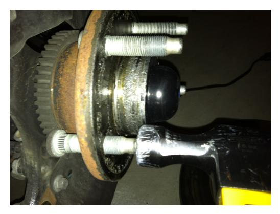
Note: This is where you will need to use the punch to remove the studs if you have any that are broken off.
