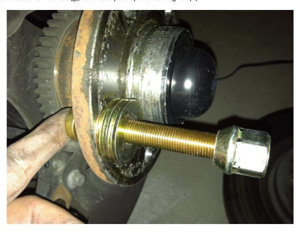
4. Take Impact Wrench (j) and corresponding Impact Socket (i) and tighten to pull the first stud through until base of the stud is tight against the back of the hub.
