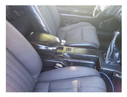
**2.** Take your plastic trim tool (or very small flat head screw driver) and very carefully put the tool under the end of the access plug and lift up. Do not use too much force because you do not want to break them.
