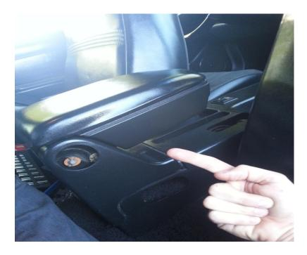
**6.** To put the center console back in you need to put the bottom in first. There are three tabs that need to go into the holes first, then you can put the top side in.
