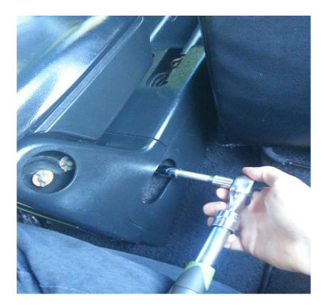
**5.** To take the center console out, you must simple pull back toward the rear of the car and lift up at the same time. It should come right out.
