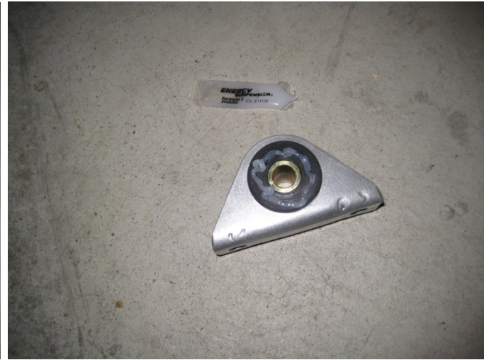
Figure 7: Greased Swaybar Bracket Bushing
