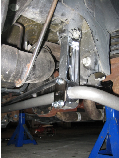
Figure 12: Swaybar Links Installed
