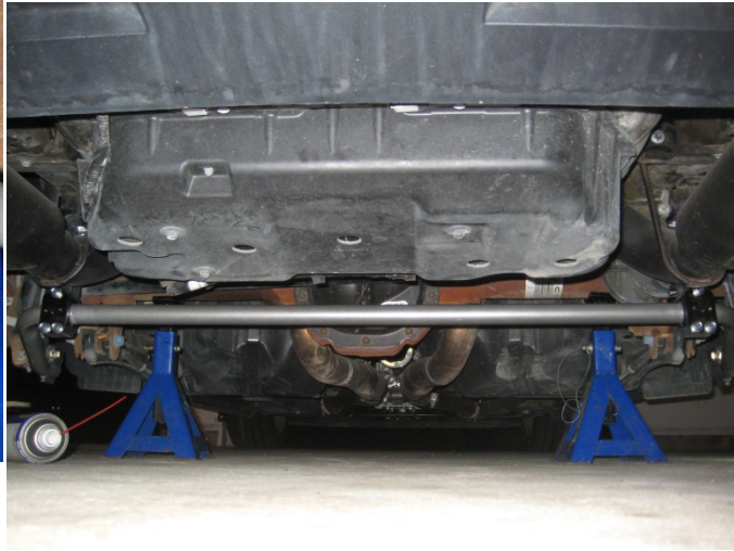
Figure 13: Steeda Swaybar Installed
