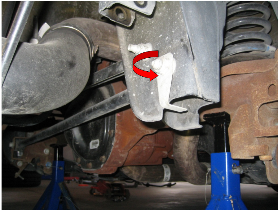
Figure 5: Panhard Bar Bolt Orientation
