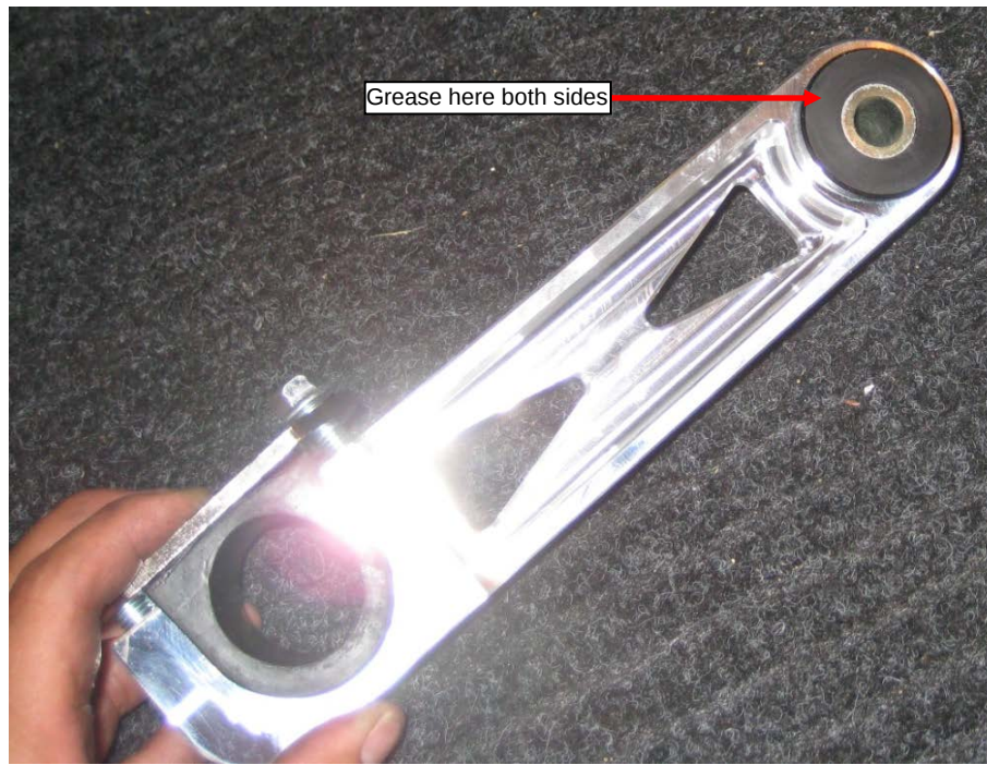
Figure 9: Swaybar link and bushings
