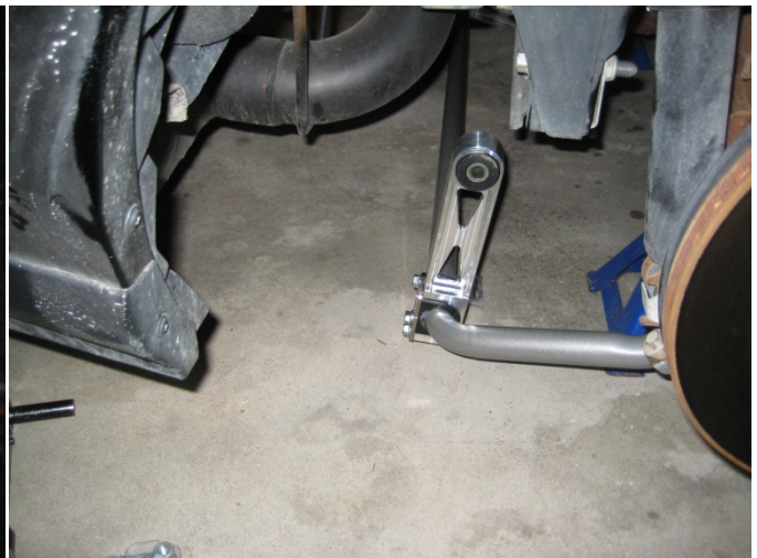
Figure 11: Steeda Swaybar Links Installed
