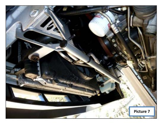
9. Using the provided zip ties, secure the lines that you removed from the factory support to the Steeda support.
