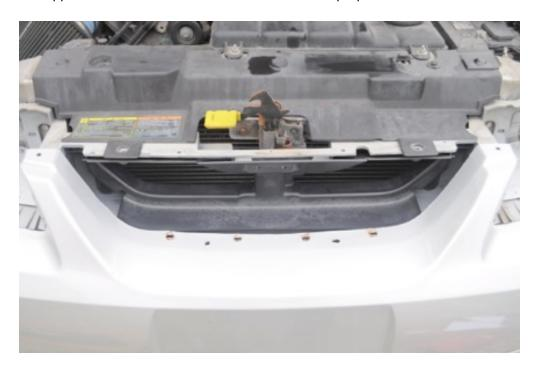
**7.** Before installing the delete kit prep the area for the pony installation by drilling or cutting a hole into the backing piece that will secure the bottom tab on the pony in place.
