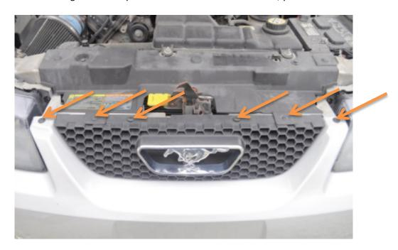
**4.** The next step is to remove the (4) 7mm bolts that hold the honeycomb down at the bottom of the honeycomb. Be patient with this process as it can be frustrating. You can view and remove these bolts by tilting the factory grille forward.
