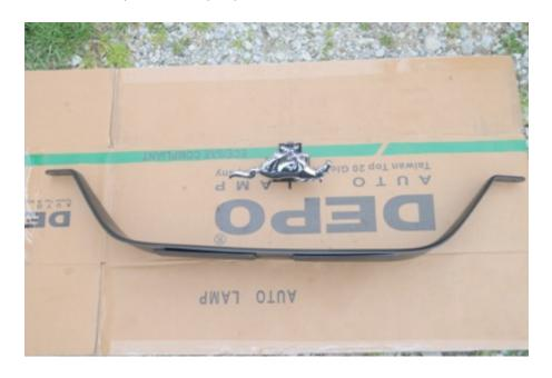
**3.** To start, locate the (4) retaining screws on the top of the factory grille along with the (2) retaining screws that retain the stock fascia. After you have located these screws remove them using the Phillips head screw driver, the flat head screw driver can assist in removing these if they are stubborn. Set the screws aside, you will re-use them later.
