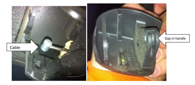
**11.** Put your new handle into place and install opening cable and reinstall the spring. There is a small recess cut into the door handle that you should place one of the ends of the spring into in order to keep it aligned properly.
