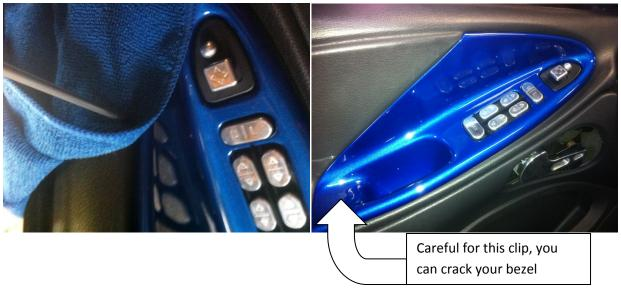
**2.** Take out the 2 retaining screws located behind the arm rest switch control plate.
