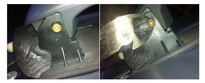
**9.** Before removing the old handle, note the direction and orientation of the old spring, which we will reuse. Remove the spring, and make sure to put it somewhere you will not lose it.
