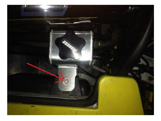
7. Fill new power steering tank with power steering fluid 1/2 inch from the top.
