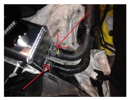
6. Install single bolt on new power steering tank. Tighten using 8MM wrench/socket.
