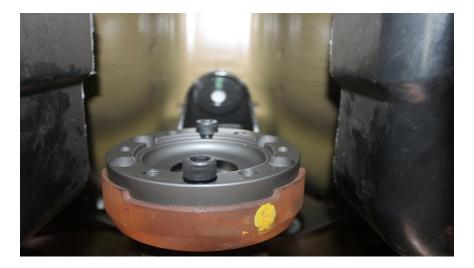
17. Install pinion flange end of new drive shaft first. Align the shaft with the screw holes and loosely put in 2 long Allen head with 8mm Allen head socket to hold rear end of driveshaft in place.
