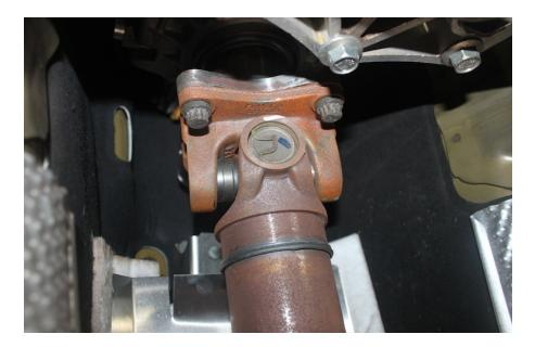
8. The middle of the drive shaft is held on by a factory safety loop with two bolts. Use a 13mm socket with an extension to remove the two bolts.
