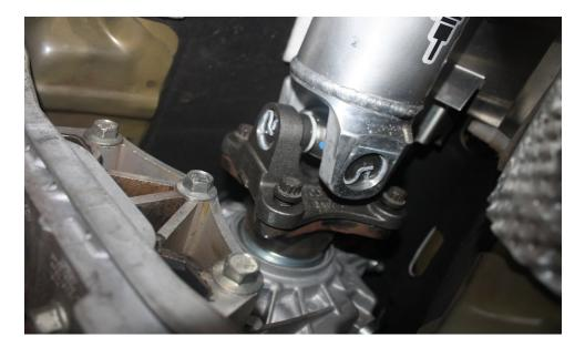
14. Place car at ride height after all bolts torqued and check the distance shown below. This distance must be between 3-1/4" and 3-3/4". If any longer or shorter, do not drive the car. Call the manufacturer for instructions. If within spec, you are good to go. Note: I have the Ford Racing T-springs (M-5300-T) with a stock upper control arm (non-adjustable) and I was still within the above specifications.
