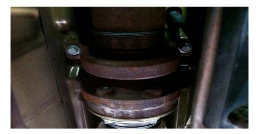
10. Go to the rear end of the car. Loosen bolts on pinion flange with breaker bar using 10mm socket. (Using an impact wrench will help for this step since the stock bolts have thread locker.)
