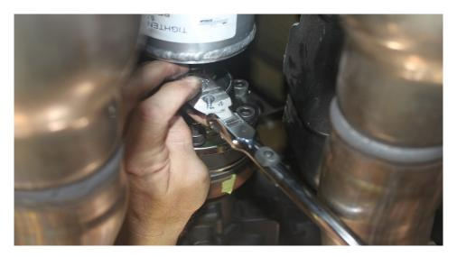
15. At transmission flange end, remove one bolt at a time, apply blue thread locker, and reinstall bolts. Tighten all four bolts and torque to 76 ft-lbs using 12 point 12 mm socket.
