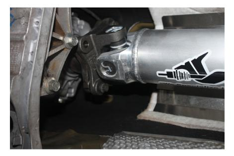
12. Put in all 6 pinion long Allen bolts, finger tight on rear end side.
