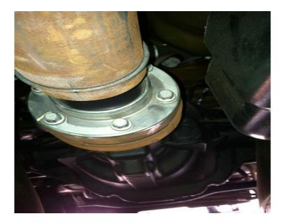
12. Go to front of car and remove final bolt on the transmission flange. Use pry bar to remove the driveshaft off the flange. Once that is done pull the driveshaft toward the rear end of the car.
