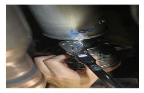
11. Next align the front end of driveshaft at the transmission flange screw holes and loosely put in the 2 stock bolts finger tight.
