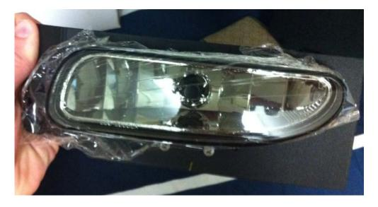
New light with plastic covering Make sure you leave the black back plastic in place when installing.
