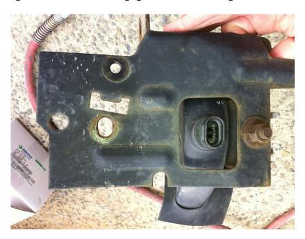
**NOTE:** At this point in your build you should check the mounting bracket and bolts for any rust or damage. I recommend that you replace the bolts that go through the fight light that mounts them to the bracket.
