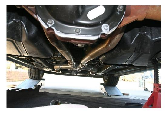
7. Compare the stock driveshaft with the new aluminum driveshaft and notice the weight difference between the two. Take your new aluminum driveshaft and slide it in from the rear. You want the rubber slider part of the driveshaft to be in the rear of the car.
