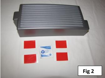
Start by removing the factory fuse box cover **–Fig 3** and clean it thoroughly using the alcohol wipe provided or a degreaser that will not harm plastics. Do not use degreaser on the finned cover as it will harm the finish. Place the urethane tape on each of the four corners of the factory cover (overlap the edge) as shown in **–Fig 4**. Let the adhesive cure for 24 hours to ensure a good bond with the factory cover.
