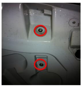
7. After the spoiler is secured, close the trunk and ensure the spoiler won't move or become loose.
