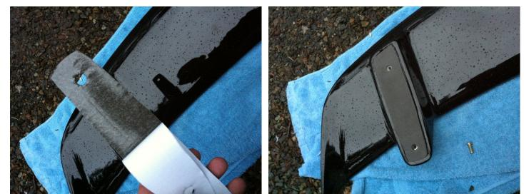
4. Remove the release paper to reveal the adhesive side of the rubber gaskets and place them on
