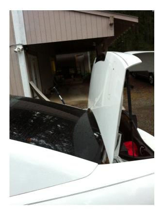
3. Remove the current spoiler. Make sure someone is holding the spoiler so it doesn't fall and damage your rear window. (This is a great time to clean the hard to reach areas underneath where the spoiler will go.)
