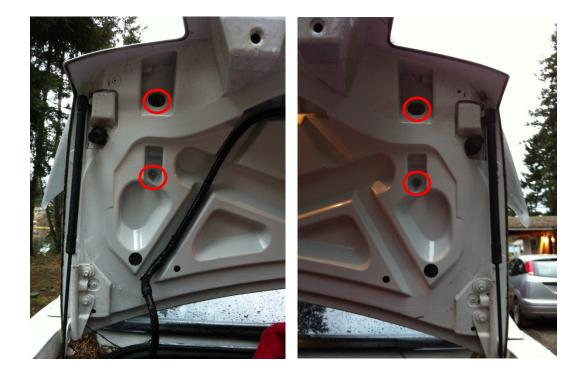
2. Use the 10mm socket wrench to unscrew the bolts on the inside of the trunk that secure the current spoiler
