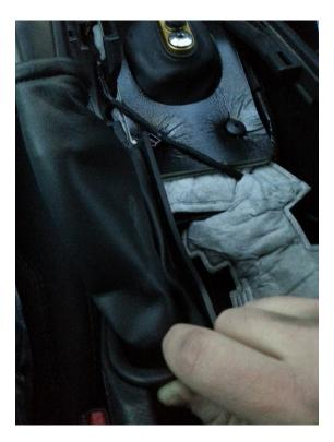
**Step 5:** Remove the factory boot from the trim ring, being careful not to break the plastic trim ring. The optional small flathead screwdriver may come in handy here. Note: The factory e-brake boot may/will tear during removal and will not be reusable due to poor quality materials. Some of the factory boot will adhere to the trim ring. Remove as much of this as possible. Do not worry if you can't remove it all, move on to the next step.
