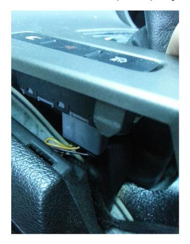
**Step 4:** Pinch the back of the emergency brake boot retainer and pull up & towards the e-brake handle to release the trim ring. Lubricate the e-brake handle with a light coating of soapy water or similar lubricant and slide the factory boot over the e-brake handle. Dry the handle with a paper towel.
