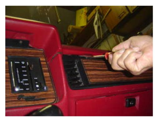
4. Remove the (2) dash pad screws located behind the instrument panel: (1) toward the center of the car on the right of the steering wheel, (1) toward the door on the left side of the steering wheel.
