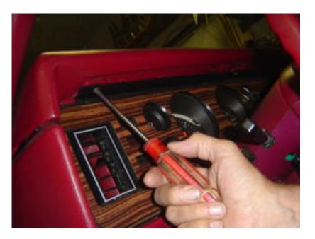
3. Remove the (2) dash pad screws on the passenger side that are at about a 45° angle.
