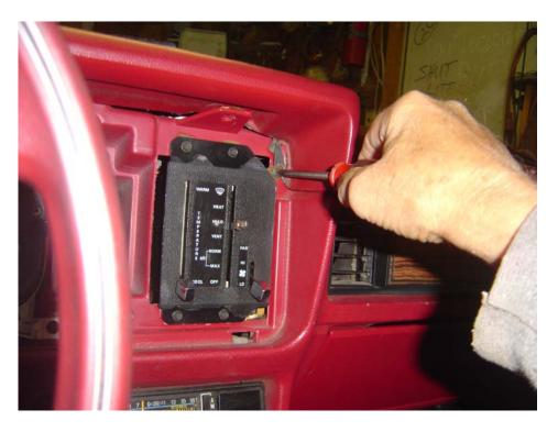
5. Lift and firmly pull the old dash pad out.
