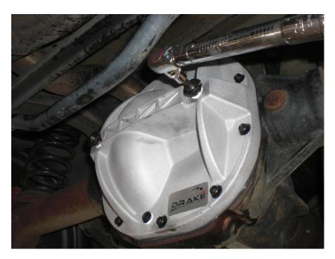
16. Holding load bolts in place, tighten jam nuts enough to keep load bolts from moving.
