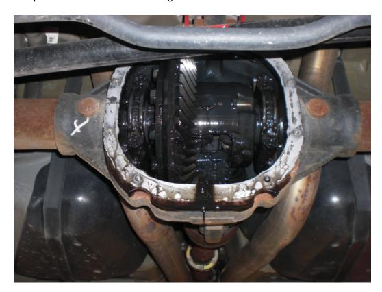
9. Using scraper, remove all gasket material from the mating surface making sure no material is left inside the housing.
