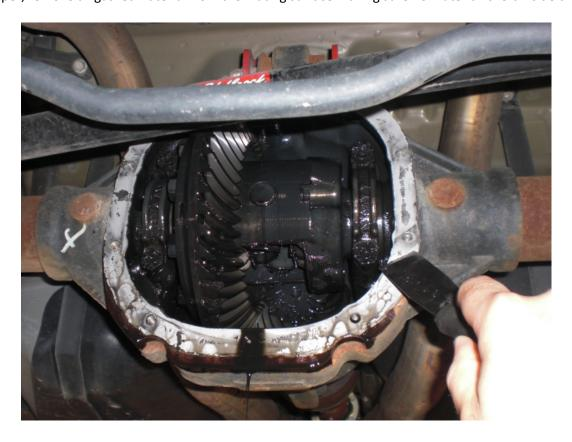
10. Make sure the load bolts are backed out completely so they do not make contact with bearing caps.
