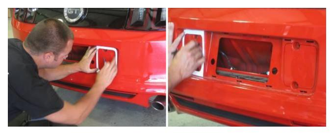
7. Using a Step Drill or similar, drill the 4 corners on both Driver and Passenger sides as shown. Caution: Make sure all wires are out of the way.
