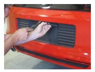
3. Remove original License Plate Panel. Insert a small hook tool into the holes used to retain the License plate. Grip firmly and pull swiftly to dislodge the molded retainers from the Fascia.
