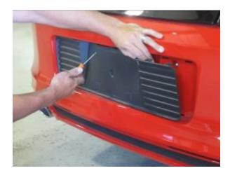
4. Use Fork Tool to release wire harness from back side of License Plate Panel.
