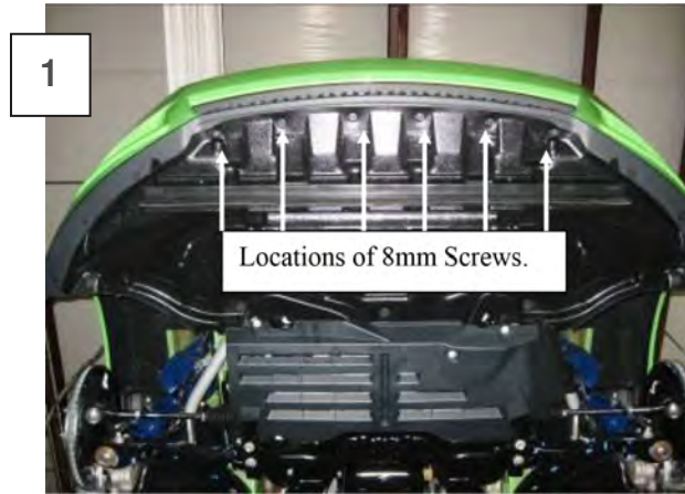
1. Remove the (6) 8mm screws that secure the center section of the factory splitter.
