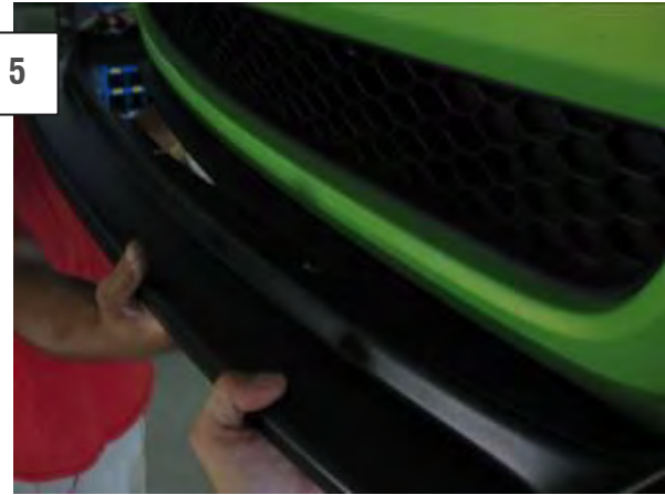
5. Place the center portion of the chin spoiler between the bottom of the fascia and the factory splitter.
