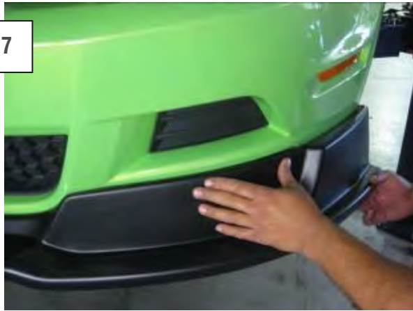
7. After the chin is in place as shown in the image below, completely remove the 3M backing and firmly press the chin to the fascia to activate the adhesive of the 3M tape.
