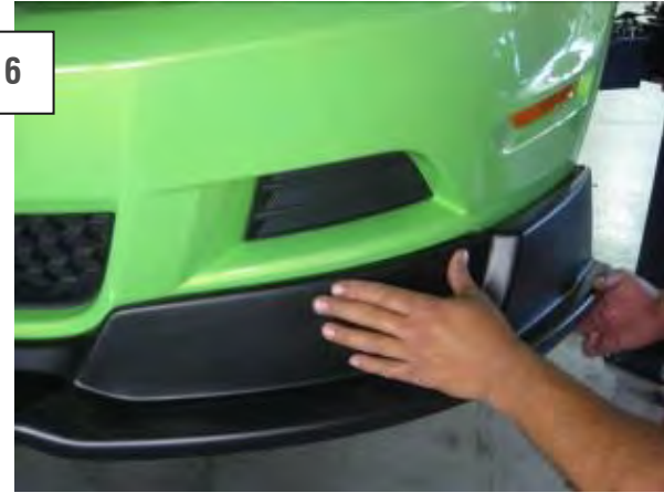
6. Peel the red backing off the 3M tape (pre installed on the chin spoiler) to create pull tab.
