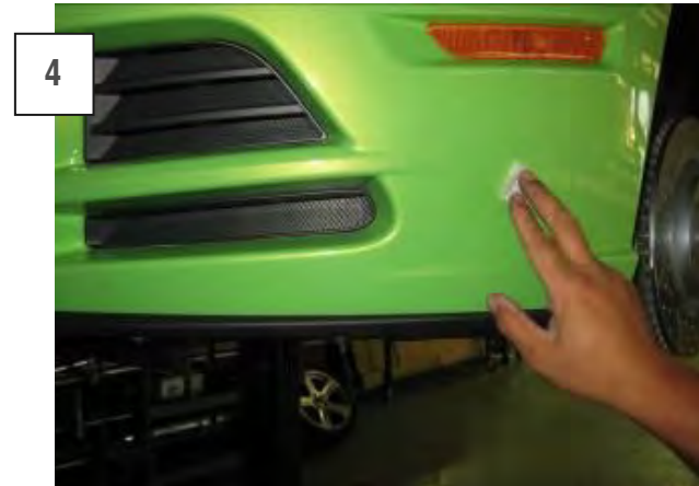
4. Clean the fascia / chin spoiler bonding surfaces with the supplied alcohol packs. Allow the alcohol to dry, then apply the 3M adhesion promoter. NOTE: Do not apply adhesion promoter above bonding area; it will leave a visible residue. Excess can be cleaned off with wax and grease remover if needed.
