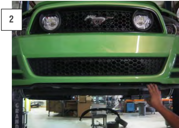
2. Pull down on the factory splitter to separate it from the fascia. NOTE: The splitter will not be removed. Your RTR chin spoiler will fit between the fascia and the splitter.
