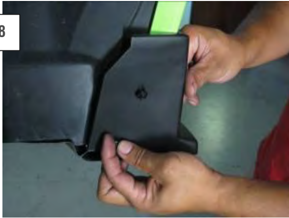
8. Reinstall the 7mm screws that were removed in step #3.
