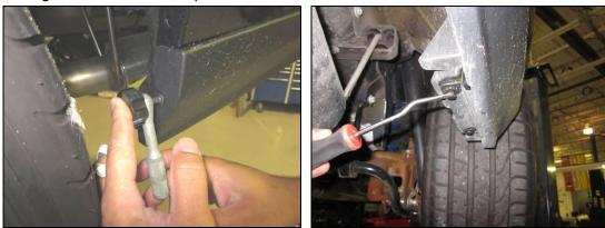
8. Under vehicle, release two white retainers found near the center attaching lower valance to underside of car (circled). Clips will likely break; they will **not** be reused.
