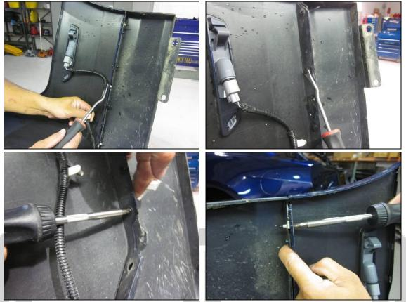
14. Left and right sides of the lower valance should now be fairly easy to separate from fascia by stretching the two gently apart. Use a fork tool if necessary to guide locking tabs out of position. Use fork tool to gently open slots in center of valance (behind license plate) to release tabs; remove valance from fascia.
