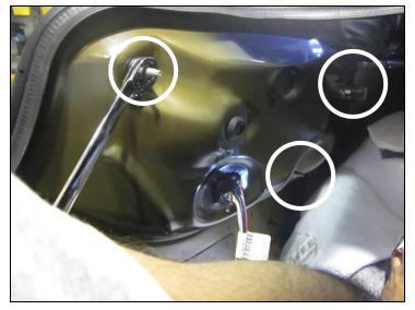
5. Locate wire harness along rear of trunk that feeds rear fascia. Disconnect electrical connector located just right of center and dislodge retainers w/ a fork tool that retain wire harness to body. Push wire grommet through body.
