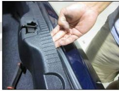
3. Disconnect the taillight harnesses (circled); push the rubber grommets through the sheet metal with your thumb, towards the rear of the car.
