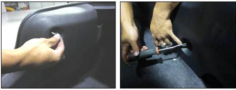
2. There are two hidden fasteners and locating pins located beneath the top of the trim panel. Using hands, carefully lift upward and forward on the panel, releasing the fasteners. Use caution as trunk courtesy light is attached to panel and wire harness has limited length. Lean panel forward in trunk; it does not need to be completely removed; only need to gain access to taillight mounting bolts.
