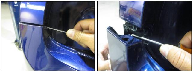
12. Four large push-pin type retainers remain at the center of the fascia (circled). With the use of a friendly assistant (one person per side of fascia), secure fascia so that left/right ends will not hit quarter panels during removal process. With free hands, pull fascia swiftly rearward to dislodge 4 remaining fasteners. Guide previously disconnected harness through hole as you remove fascia from car. Place fascia on soft surface.
