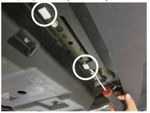
9. Just inboard from exhaust tips, locate two black plastic "straps" (one per side) that connect lower valance to car. These extend vertically to body, next to exhaust hangers. Each is fastened to car w/ a push pin, release using panel/fork tool.
