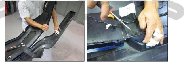
15. Install RTR Diffuser/Splitter to rear fascia, reversing the procedure outlined above. Begin by installing all locking tabs of diffuser/splitter into rear fascia, pressing firmly in place with thumbs. Reinstall push pins, screws, and push pin wire harness retainers. Once complete, turn fascia over to inspect and ensure all tabs have been properly seated. Note locating pins on fascia (circled below).
