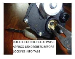
(9A)Still using the needle nose pliers pull upwards slightly locking it in place. Install the black plastic cap (removed in step 5) it only goes on one way.
