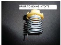
(7)The curved spring end goes into the plastic gear on the new TB. Hold the TB upright (important) with the spring and white cap on the TB plastic gear.
