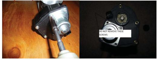
(3) On the throttle body that was removed, remove the TPS sensor located on the left side of the TB. Remove the 2 torx screws that attach the TPS to the TB. Then remove the TPS sensor.
