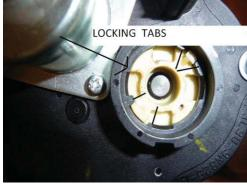
(10)Install the new TB, reverse the procedure used to remove the TB, reinstall the intake assembly.
