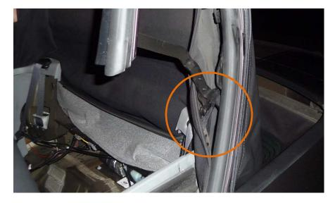
• Using the included Velcro straps, tie the elastic band closer one of the support bars
