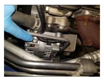
9. Crawl back underneath. Remove the 10mm nut that secures the power steering line to the single 15mm lower mounting bolt for the alternator. Remove that 15mm alternator mounting bolt. Once this bolt is removed, the alternator will be free hanging. Tilt the unit backwards and counterclockwise about 20 degrees and it should slide out.
