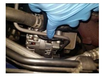
8. Unthread the x2 15mm alternator mounting bolts. They are long will not be fully removed until the alternator is fully out from under the vehicle. Use a ratcheting box end to maximize your time.
