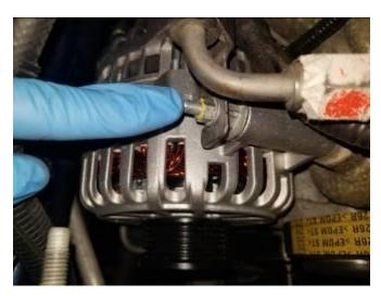
10. Once the alternator is removed, the upper bolts are available to be fully removed. Install them into the corresponding holes in the new alternator.
