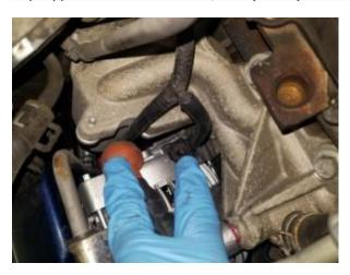
5. Remove the x4 (15mm) bolts holding on the sway bar to the front support. Once loose, pull it forward and let it hang to make room for the alternator to drop out.
