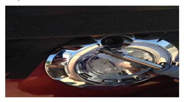
6. If the emblem doesn't want to budge then heating it with a hair dryer may be a way to loosen the adhesive on the back of the emblem.
