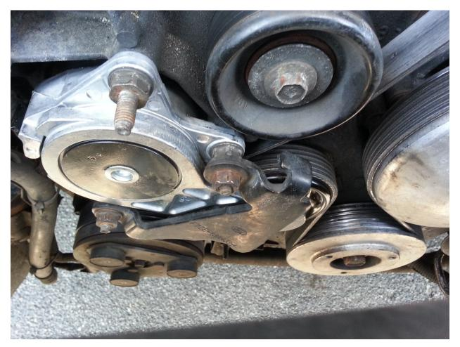
1. Remove the 2 nuts on the right and bottom holding the bracket (if you have one) covering the belt tensioner hole with the ½"inch socket. They will rotate counter clockwise. Once the nuts are removed the bracket will pull right off.
