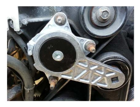
9. The belt tensioner should now easily just pull right out. You can see where my old tensioner pulley started going bad and was rubbing up on the engine. (Hold the belt up as you pull the tensioner out because the pulley will be coming out to and you do not want to belt to come off the other pulleys.)
