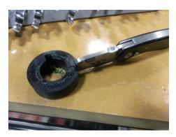
7. Now, slide the thin metal piece of the bushing assembly onto the snout of the shifter.
