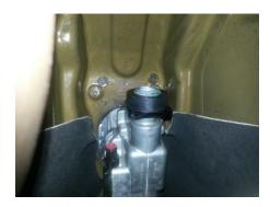
Slide the thicket part of the bracket over the bushing, mate it with the rear plate, and bolt the assembly back together.
