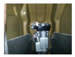
10. Reinstall the (2) 10mm nuts and tighten the assembly to the vehicle.
