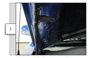
Making sure the hood is properly supported by the factory prop rod, remove the forward most bolt on the hood hinge.
