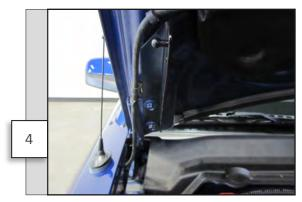
Loosen the rear most bolt on the hood hinge just enough to slide the larger bracket (marked P-U) in between the hood hinge and bolt. (do not install the bracket between the hood hinge and hood)
