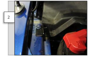
Install bracket marked P-L using factory fender bolt as shown.
