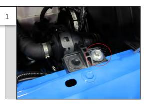
Remove the bolt holding the canister bracket to the inner fender. Also remove the factory u-nut from the fender for reuse.
