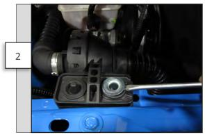
Using a flat head screwdriver or trim removal tool, pry the metal bushing from the bracket as shown.
