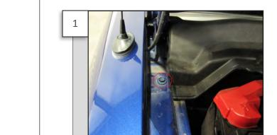
Prop hood open and remove the fender bolt shown below.
