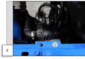
Re-insert the metal bushing (removed in Step 2) into the bottom right side of the bracket and re-install assembly on the bottom side of the inner fender using the original hardware (removed in Step 1).
