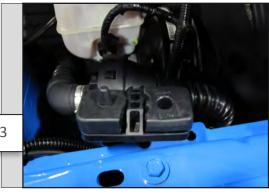
Remove the square rubber bushing from the bracket and cut ½" from the center of it. Place the two halves of the bushing onto the top side of the bracket as shown.
