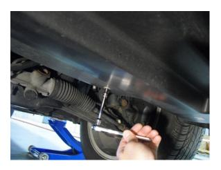
**Step 2:** Place the four included U-Clips over the four included J-Hooks as shown.
