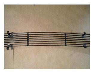
**Step 4:** Place the billet grille over the factory grille. From underneath the car, adjust the J-Hooks to wrap around the factory plastic grille as shown.
